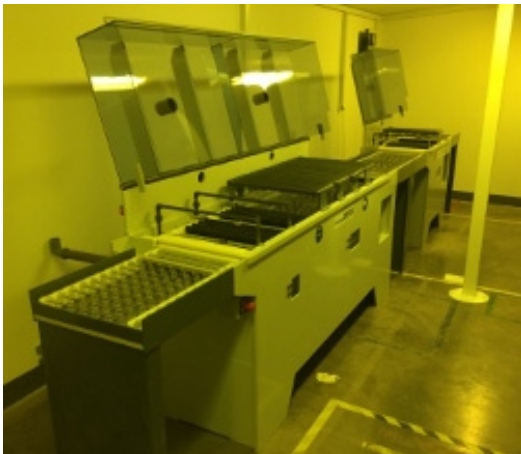
Production line made from a SPRINT 4500 for developing and a SPRINT 4500 for etching with 4 times enlarged etching area
